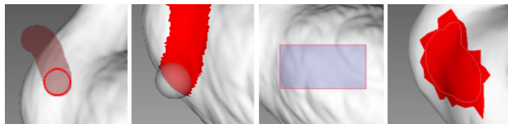
Figure 8.13.: Various Eraser modes (from left to right): 2D , 3D , Rectangular , Lasso .
