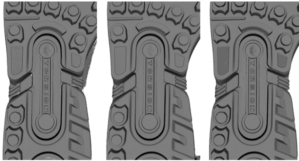
Figure 8.38.: Models of a shoe sole obtained using various algorithms: Fast fusion (left), Smooth fusion (middle) and Sharp fusion (right).
