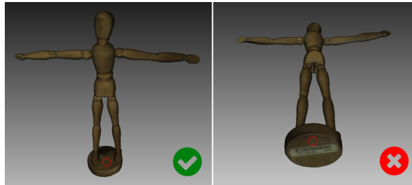
Figure 8.15.: Selecting a flat region in the Cutoff-plane selection mode.
