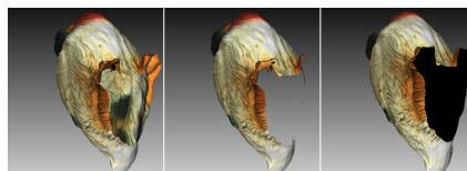
Figure 6.10.: Examples of different methods for back-face rendering. Show back-face mode on the left, hide ( Cull ) in the middle and Black on the right.
