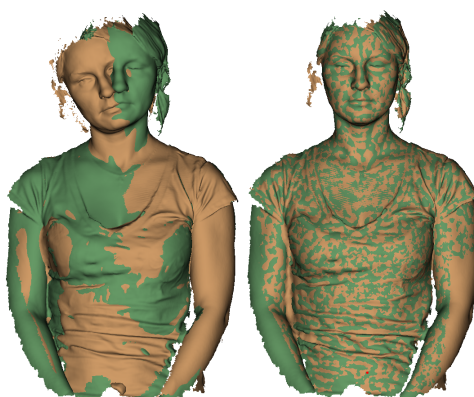
Figure 8.30.: Two models after rigid (left) and nonrigid alignment (right).
