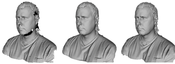
Figure 8.37.: Models of a human subject obtained using various algorithms: Fast fusion (left), Smooth fusion (middle) and Sharp fusion (right).
