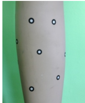
Figure 5.9: Non-coded targets placed on an object.
