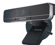
Figure 3.8: Intel RealSense 3D camera by Creative (F200)
