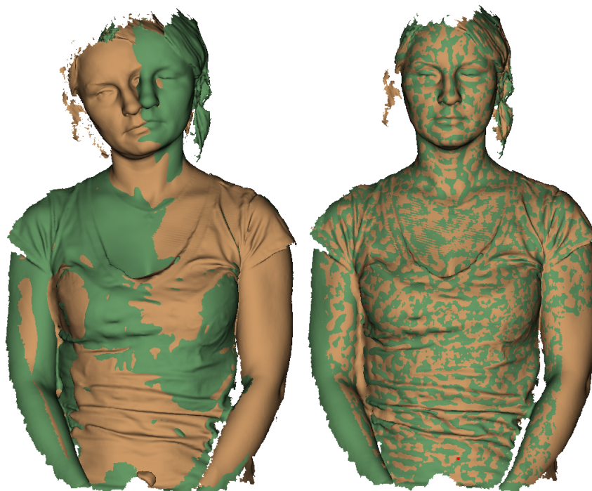
Figure 8.23: Two models after rigid (left) and nonrigid alignment (right).
