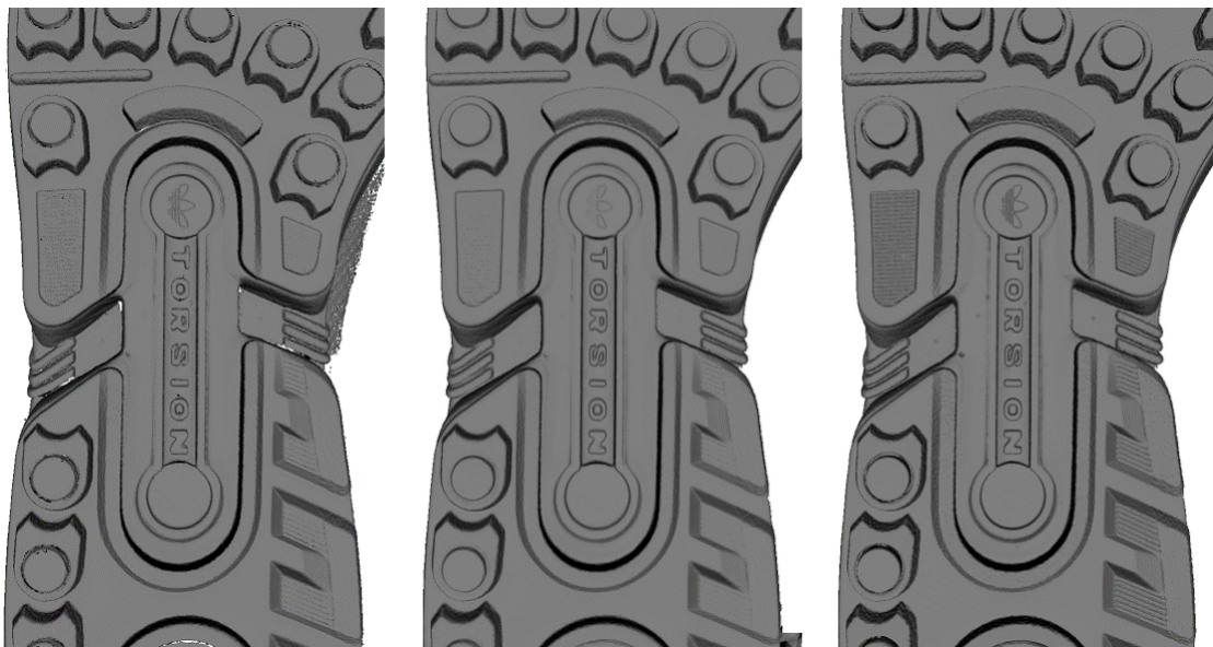
Figure 8.30: Models of a shoe sole obtained using various algorithms: Fast fusion (left), Smooth fusion (middle) and Sharp fusion (right).
