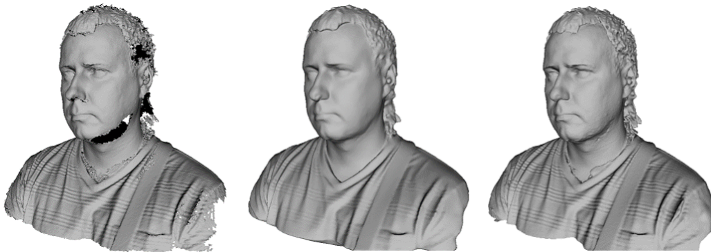
Figure 8.29: Models of a human subject obtained using various algorithms: Fast fusion (left), Smooth fusion (middle) and Sharp fusion (right).
