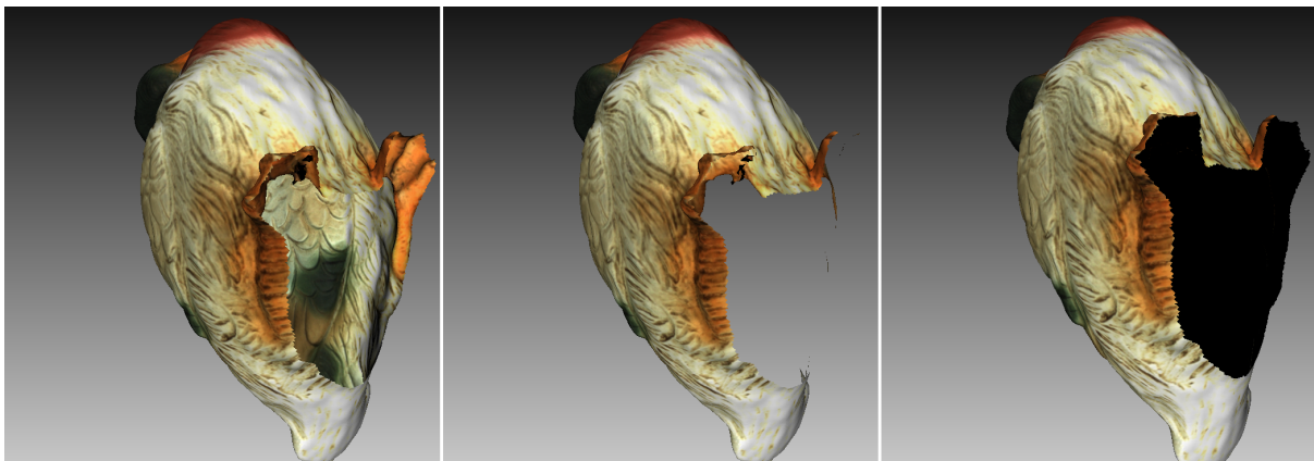
Figure 6.10: Examples of different methods for back-face rendering. Show back-face mode on the left, hide ( Cull ) in the middle and Black on the right.
