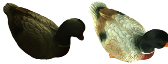
Figure 5.15: Influence of ambient light on captured results. On left: flash is turned off; ambient light is poor; results—dark texture. On right: flash is turned off; lighting conditions are improved; results—good texture.
