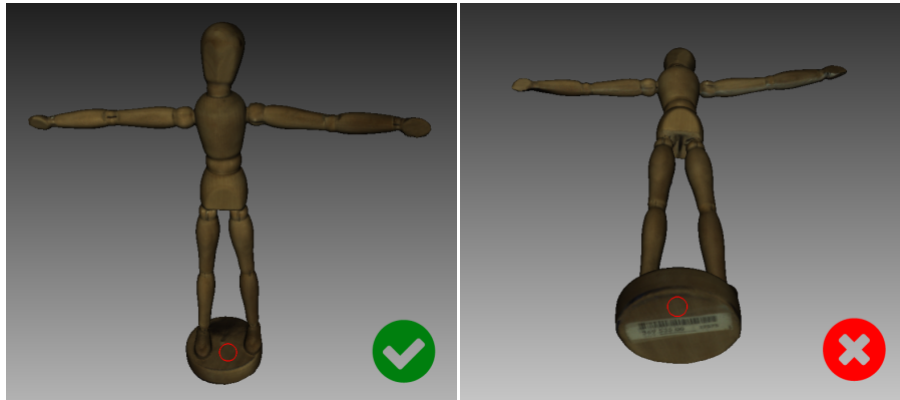
Figure 63: Selecting a flat region in the Cutoff-plane selection mode.
