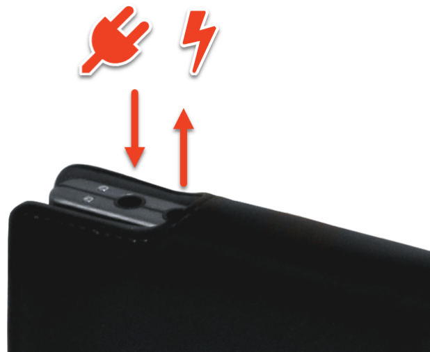
Figure 8: Battery ports from left to right: Input, Output.
