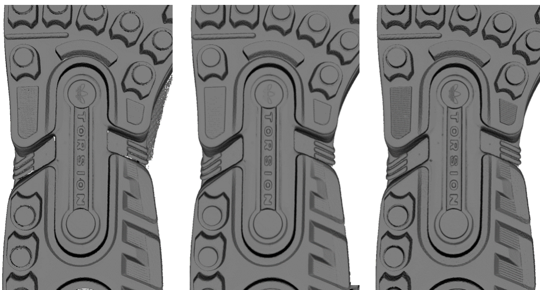
Figure 82: Models of a shoe sole obtained using various algorithms: Fast fusion (left), Smooth fusion (middle) and Sharp fusion (right).
