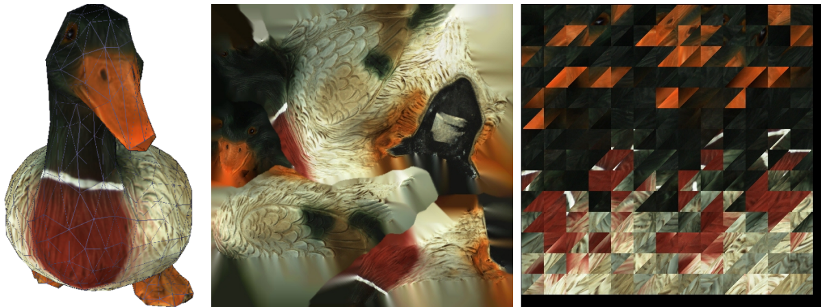
Figure 96: Texture mapping methods: mesh with texture applied (left), texture-atlas sample (middle) and triangle-map sample (right). The latter covers only a portion of the mesh surface (the rest two images not shown).
