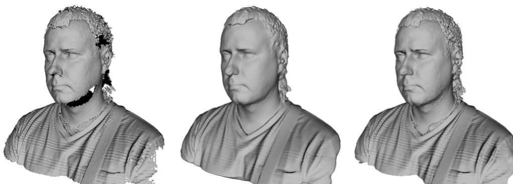
Figure 81: Models of a human subject obtained using various algorithms: Fast fusion (left), Smooth fusion (middle) and Sharp fusion (right).
