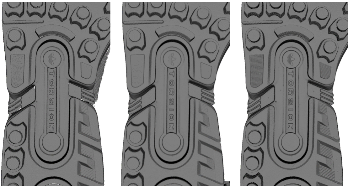
Figure 79: Models of a shoe sole obtained using various algorithms: Fast fusion (left), Smooth fusion (middle) and Sharp fusion (right).
