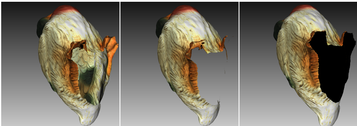
Figure 52: Examples of different methods for back-face rendering. Show back-face mode on the left, hide ( Cull ) in the middle and Black on the right.
