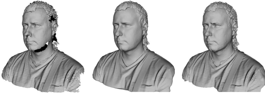
Figure 78: Models of a human subject obtained using various algorithms: Fast fusion (left), Smooth fusion (middle) and Sharp fusion (right).
