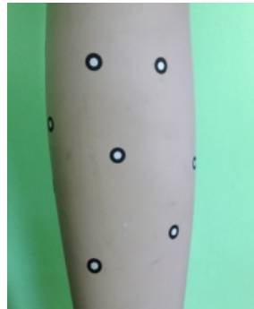
Figure 36: Non-coded targets placed on an object.
