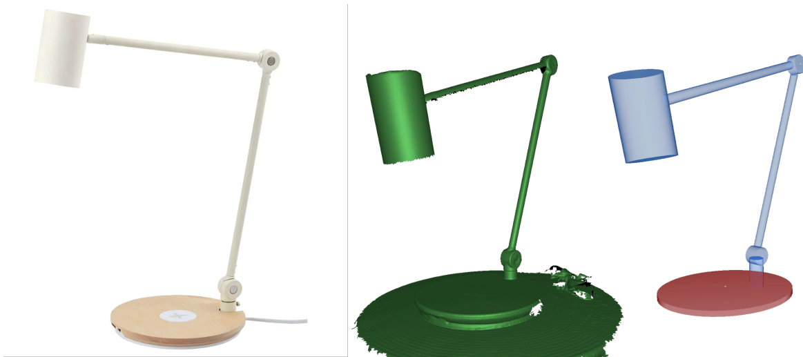
Figure 123: From left to right: original object, scanned model, a set of constructed primitives.
