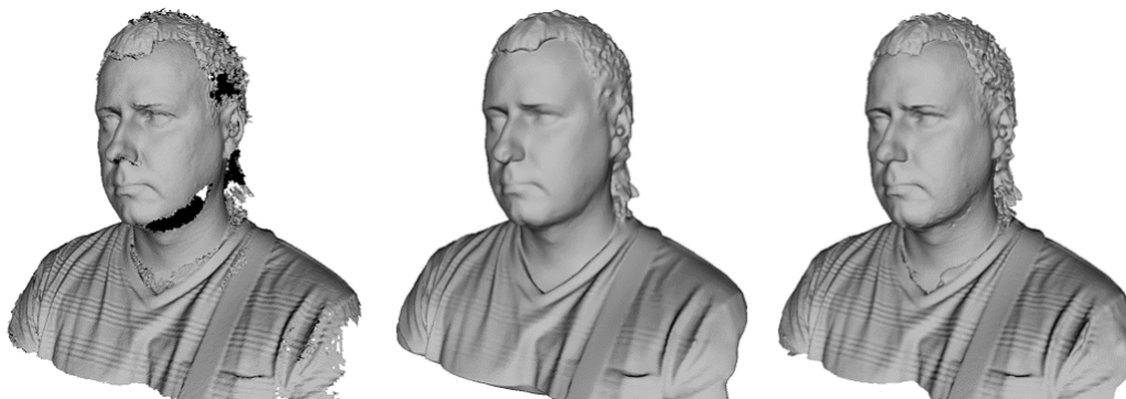
Figure 91: Models of a human subject obtained using various algorithms: Fast fusion (left), Smooth fusion (middle) and Sharp fusion (right).
