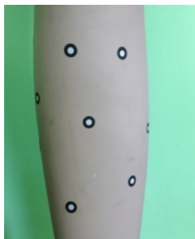
Figure 46: Non-coded targets placed on an object.
