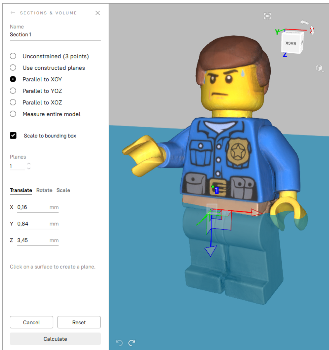
Figure 140: Changing location of a new section in the Translate mode.
