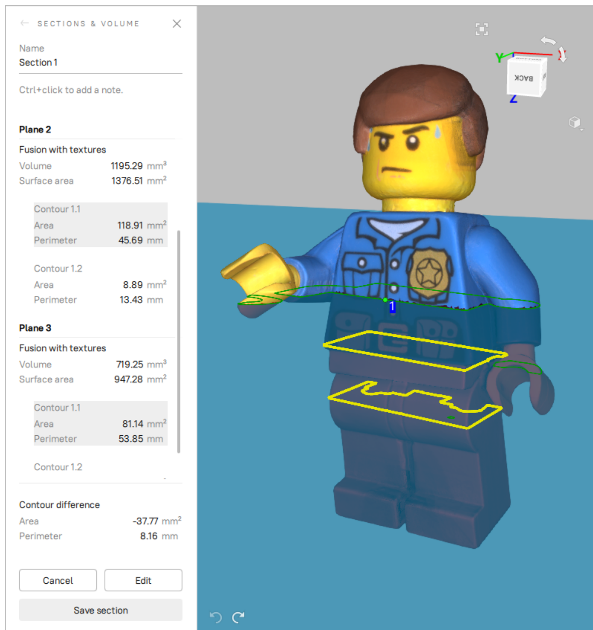
Figure 142: Calculating the contour difference.
