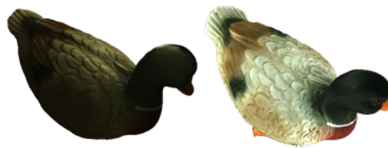
Figure 51: Influence of ambient light on captured results.
