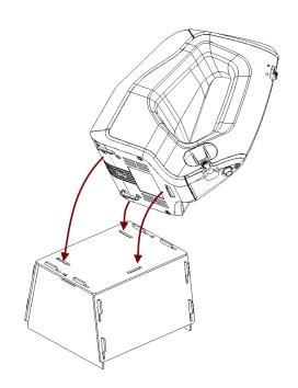
Figure 201: Placing Artec Spider on the stand
