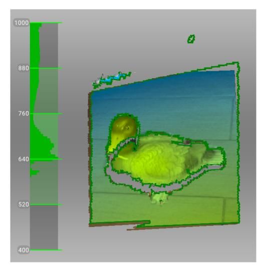
Figure 40: Distance meter and distance color showing surfaces that fall within the optimal range for Artec Eva.
