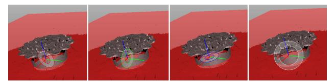
Figure 109: Various controls for orienting cutoff plane: around axes (X, Y and Z) and view direction.
