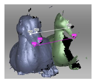
Figure 120: Before alignment: two point-set added.
