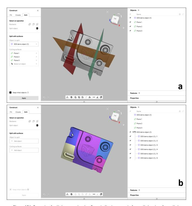
Figure 176: Example of splitting a mesh using 3 pre-built planes: a—before splitting, b—after splitting
