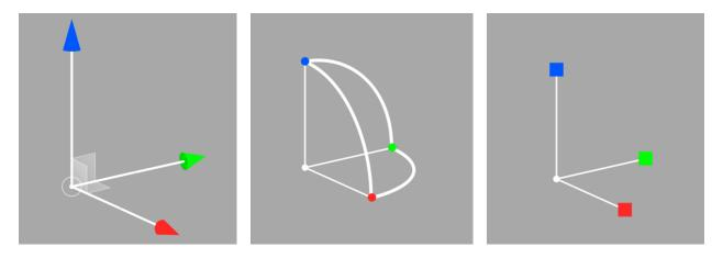
Figure 183: Gizmos for the Translate, Rotate and Scale respectively.
