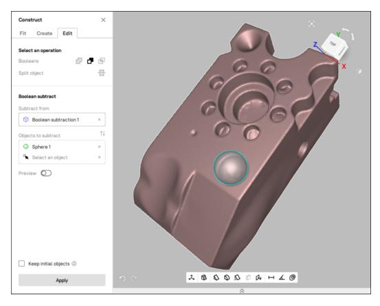
Figure 175: Selected objects are highlighted before the boolean operation
