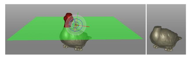
Figure 140: Applying Cutoff-plane selection in Defeature brush.
