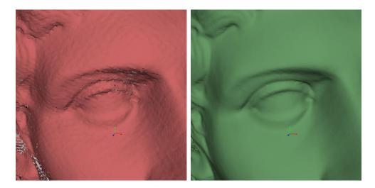
Figure 131: Surface noise caused by insufficient data (left) and improved model after adding one more scan (right).
