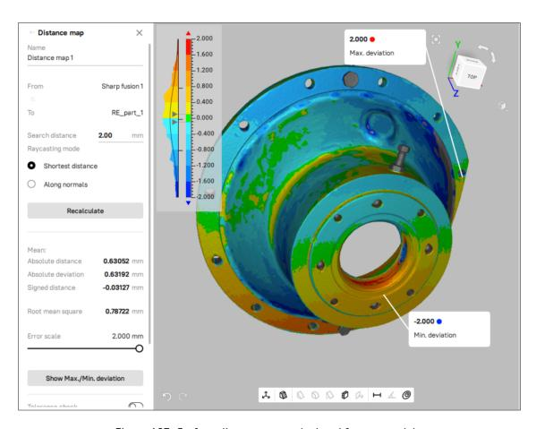
Figure 187: Surface-distance map calculated for two models.
