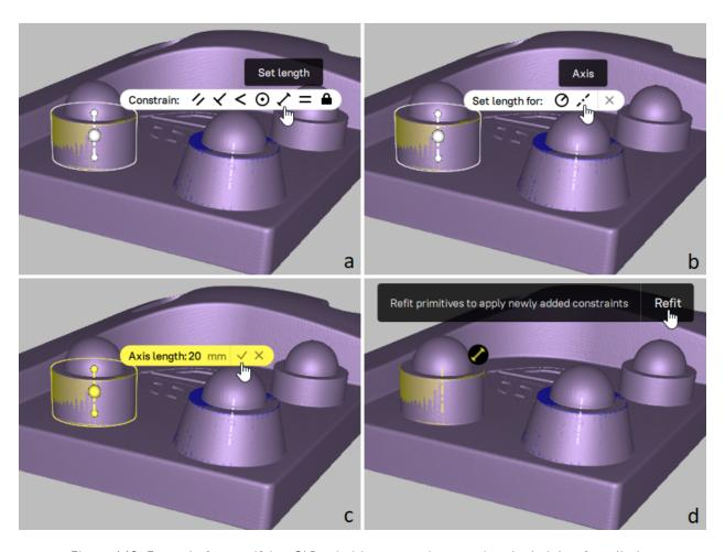
Figure 168: Example for specifying CAD primitive constraints: setting the height of a cylinder.
