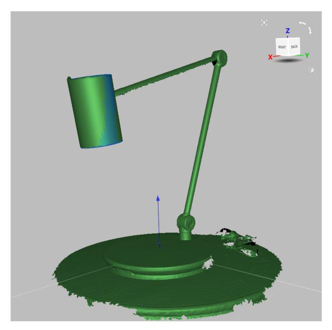
Figure 164: Cylinder (blue) fit into the model.
