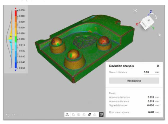
Figure 78: The Deviation analysis tool with calculated distance map
