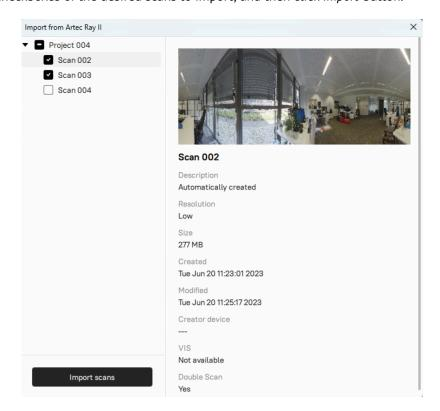
Figure 90: Dialog for importing Ray II scans from the selected project (\*.artec).
