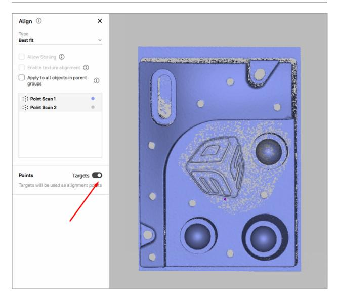
Figure 116: Alignment of Artec Point point clouds using targets.
