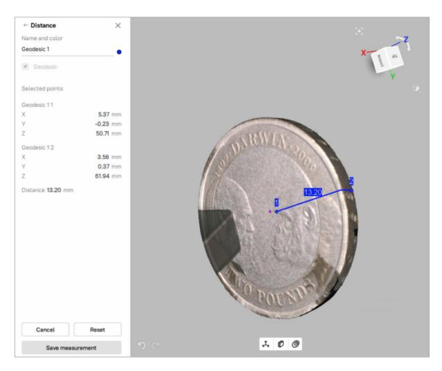
Figure 182: The Geodesic measurement.
