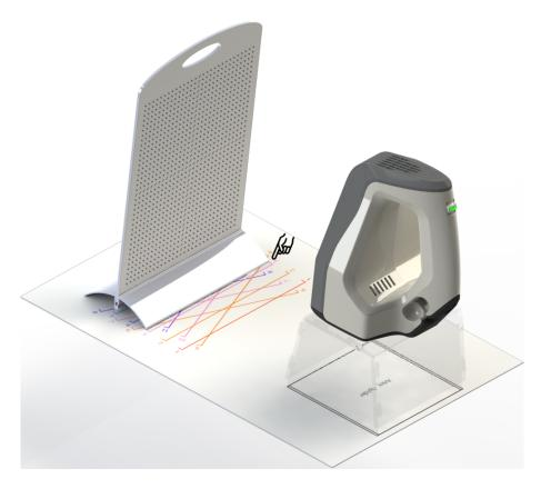
Figure 202: Calibration rig, positioning sheet and scanner stand with Artec Spider.
