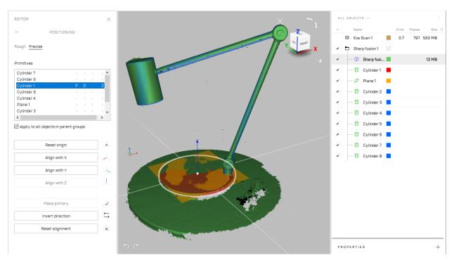
Figure 172: Editor → Precise positioning: the aligned CAD primitive is highlighted.
