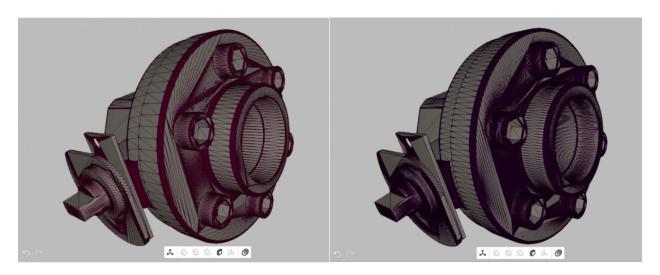
Figure 167: CAD model converted to a mesh with 72 (left) and 144 (right) accuracy values.
