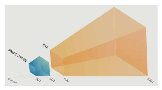
Figure 13: Fields of view for Eva and Spider 3D scanners.
