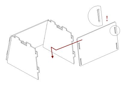
Figure 208: Assembling the back wall.
