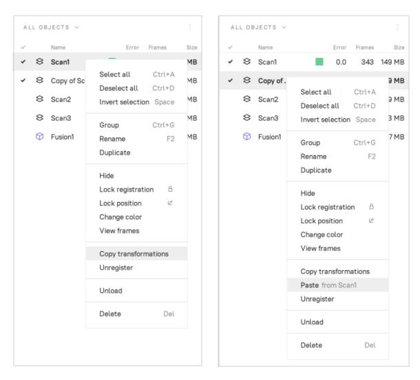
Figure 126: Transferring transformations: copying transformations (left) and pasting them (right)
