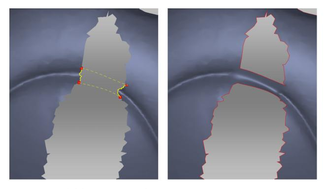
Figure 134: Specifying fragments. Correct fragments can resolve original geometry.
