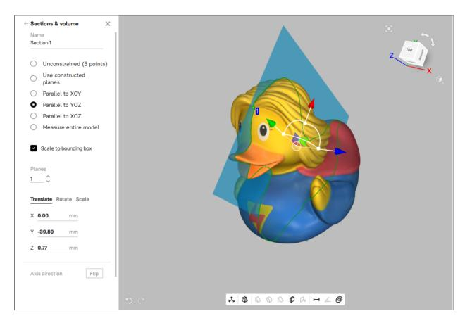
Figure 184: Change location and preview a new section by dragging the Gizmo controls.
