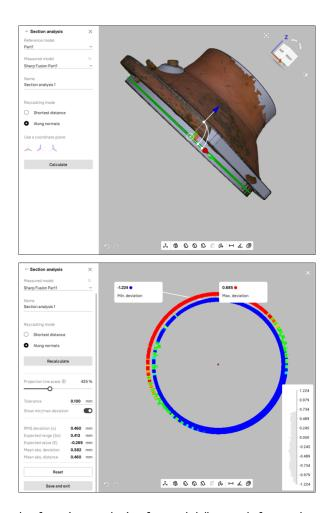
Figure 189: Result of section analysis of a model (bottom), for a selected section (top).
