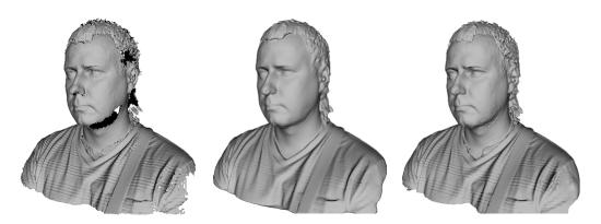
Figure 127: Models of a human subject obtained using various algorithms: *Fast fusion* (left), *Smart fusion* (smooth, middle) and *Smart fusion* (sharp, right).
