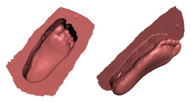
Figure 161: Normal inversion application: obtaining a foot model (right) from its cast (left).
