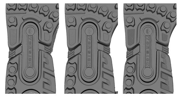
Figure 128: Models of a shoe sole obtained using various algorithms: *Fast fusion* (left), *Smart fusion* (smooth, middle) and *Smart fusion* (sharp, right).
