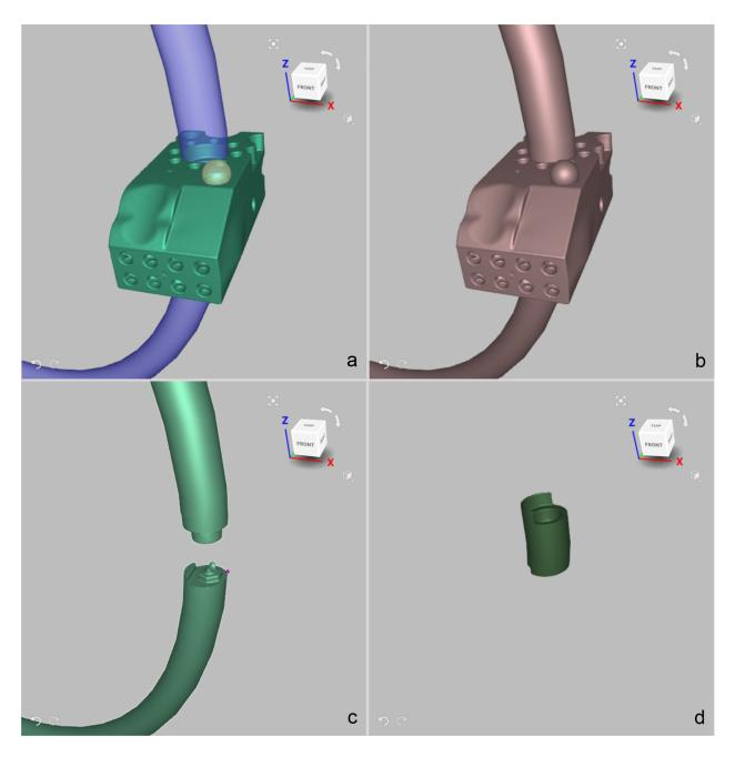
Figure 174: Examples of Boolean operations with objects: a—source objects, b—Boolean unification, c—Boolean subtraction, d—Boolean intersection
