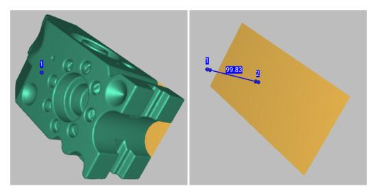
Figure 181: Thickness measurement: selecting a point on the side opposite to the plane (left), clicking the plane to determine distance to it (right).
