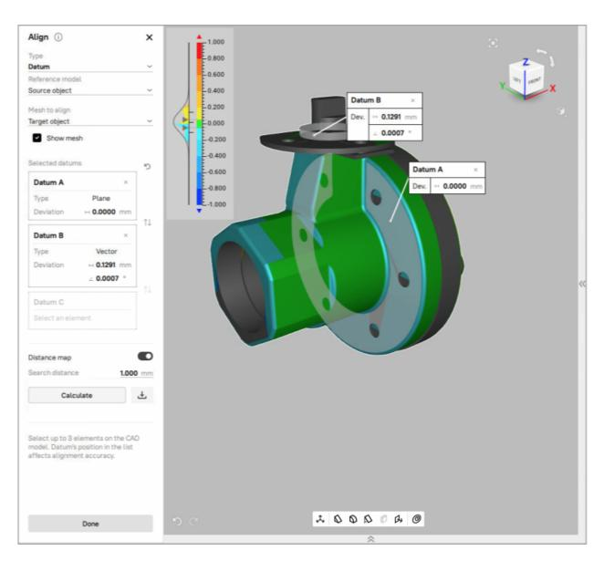
Figure 124: Example of a distance map calculated in the Datum Alignment type
