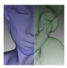
Figure 137: Mesh simplification: original mesh on the left, optimized mesh on the right.
