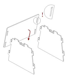
Figure 207: Assembling the front wall.
