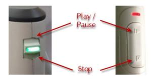
Figure 14: Scanner buttons: Artec Spider on the left and Artec Eva on the right.
