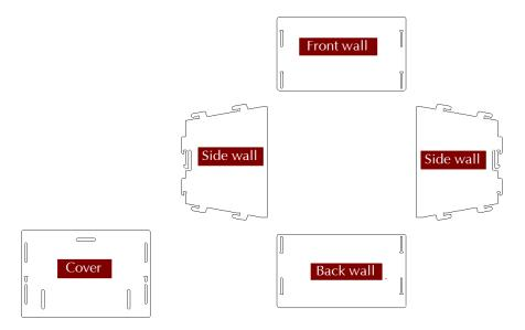
Figure 206: Parts of the scanner stand.
