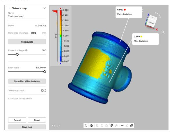
Figure 188: Thickness map calculated for a model.
