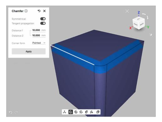
Figure 73: Chamfer with Tangent propagation parameter on
