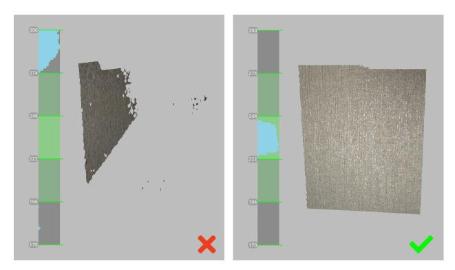
Figure 39: Scanner orientation and reconstructed surfaces.
