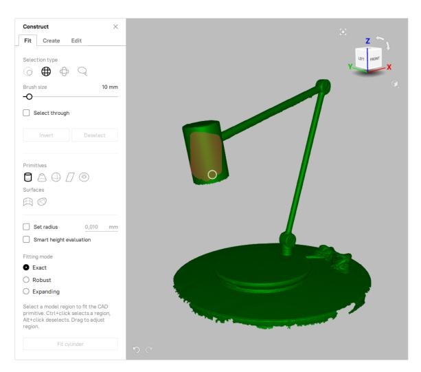
Figure 163: The Fit tab of the Construct panel: specifying the area using the 3D brush.
