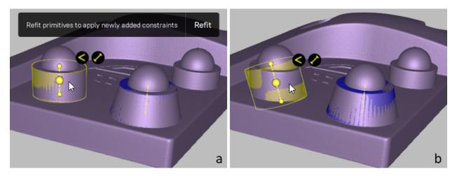
Figure 170: Example for applying CAD primitive constraints.
