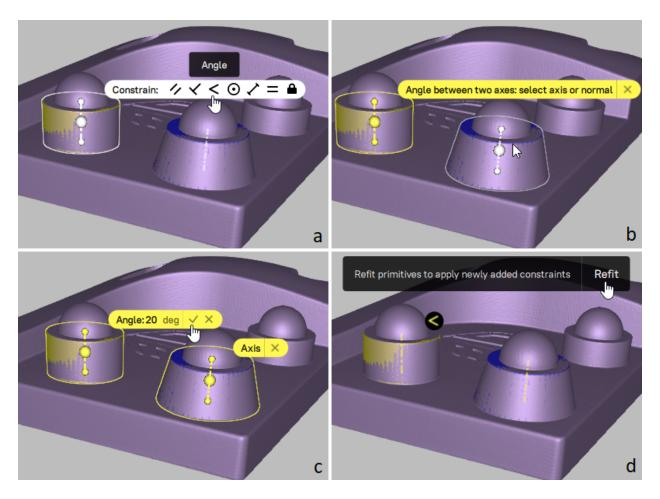
Figure 169: Example for specifying CAD primitive constraints: setting the requirement that the axes of two primitives are at a given angle to each other.
