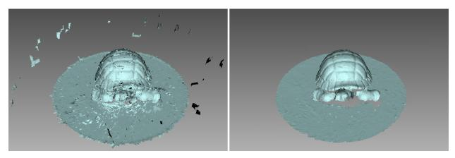
Figure 106: Outlier removal: before and after.
