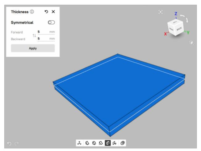
Figure 75: The Thickness tool with a 5mm forward and backward offset
