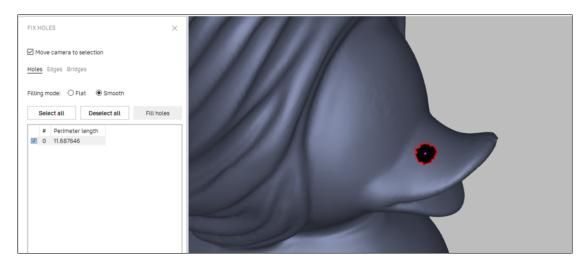
Figure 144: One hole on a curved surface, marked for correction.
