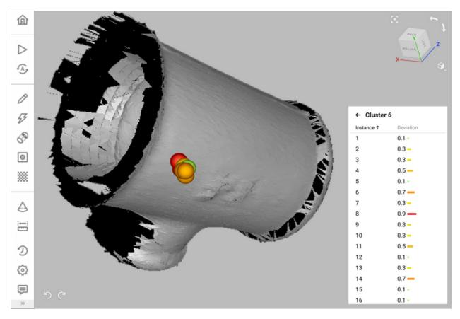
Figure 53: The list of clusters and their deviation displayed in the Features panel and in the 3D View window.
