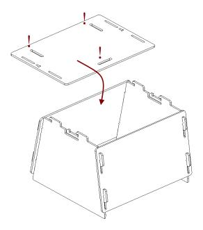
Figure 209: Mounting the cover.
