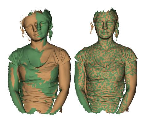
Figure 118: Two models after Best Fit (left) and nonrigid alignment (right).
