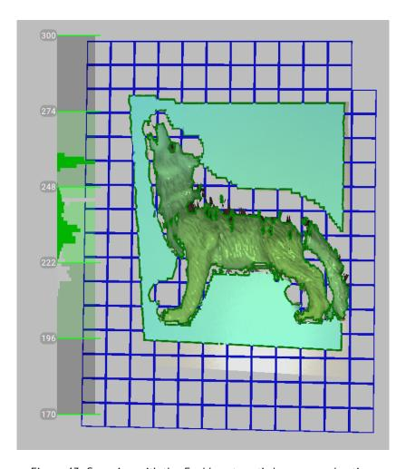
Figure 43: Scanning with the *Enable automatic base removal* option.
