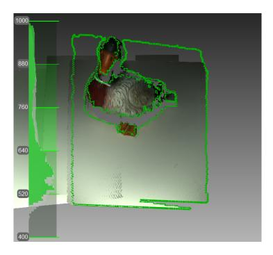
Figure 41: Texture tracking renders color object (scanner's current field of view outlined in green).
