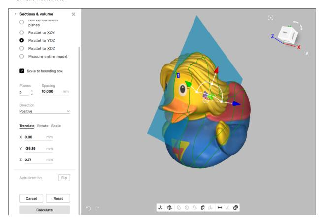
Figure 185: Calculating with two planes.
