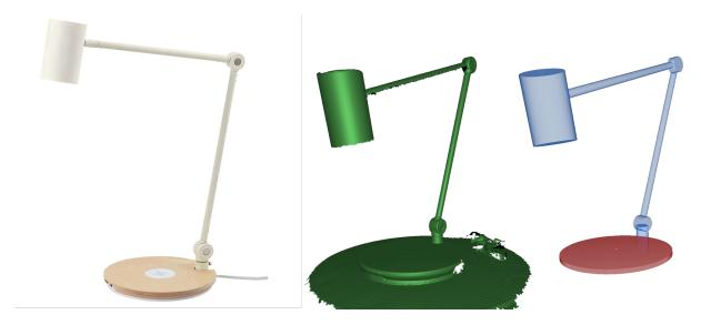
Figure 162: From left to right: original object, scanned model, a set of constructed primitives.
