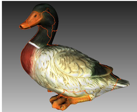
Figure 98: 3D model with texture-atlas boundaries.
