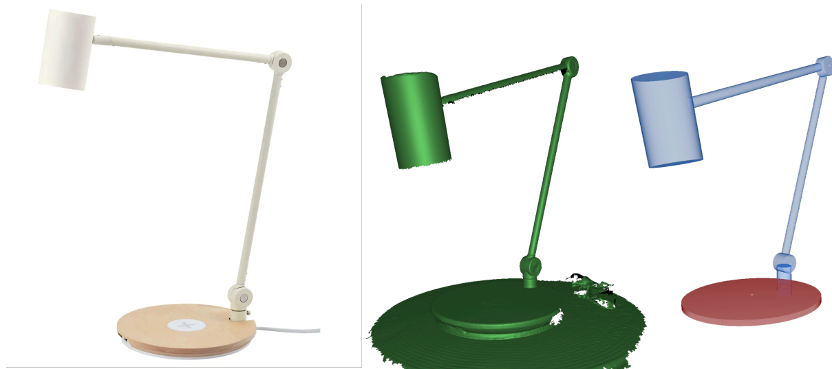
Figure 176: From left to right: original object, scanned model, a set of constructed primitives.
