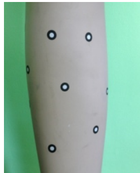
Figure 57: Non-coded targets placed on an object.
