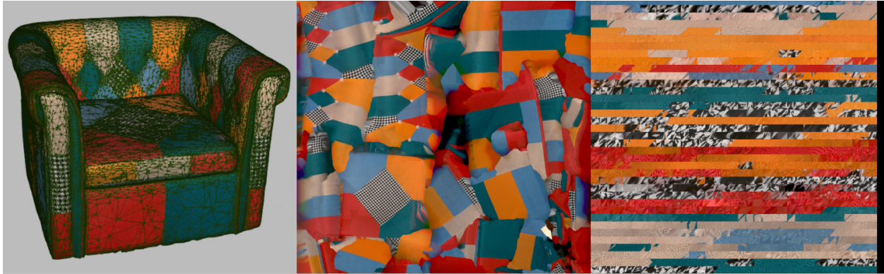
Figure 163: Texture mapping methods: mesh with texture applied (left), texture-atlas sample (middle) and triangle-map sample (right). The latter covers only a portion of the mesh surface (the rest two images not shown).
