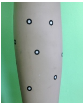
Figure 57: Non-coded targets placed on an object.
