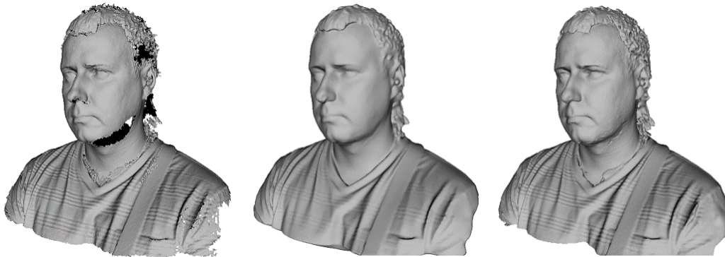
Figure 138: Models of a human subject obtained using various algorithms: Fast fusion (left), Smart fusion (smooth, middle) and Smart fusion (sharp, right).
