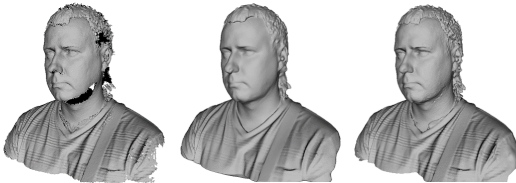
Figure 151: Models of a human subject obtained using various algorithms: Basic fusion (left), Smart fusion (smooth, middle) and Smart fusion (sharp, right).
