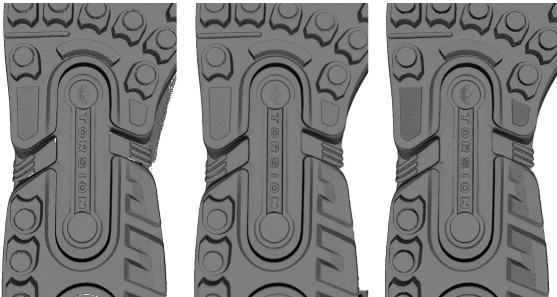
Figure 152: Models of a shoe sole obtained using various algorithms: Basic fusion (left), Smart fusion (smooth, middle) and Smart fusion (sharp, right).
