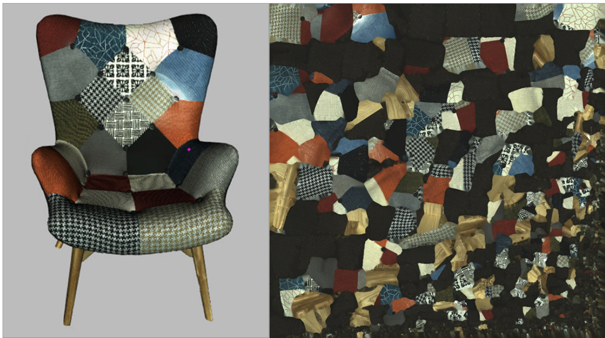
Figure 176: Texture mapping methods: mesh with texture applied (left) and texture-atlas sample (right).
