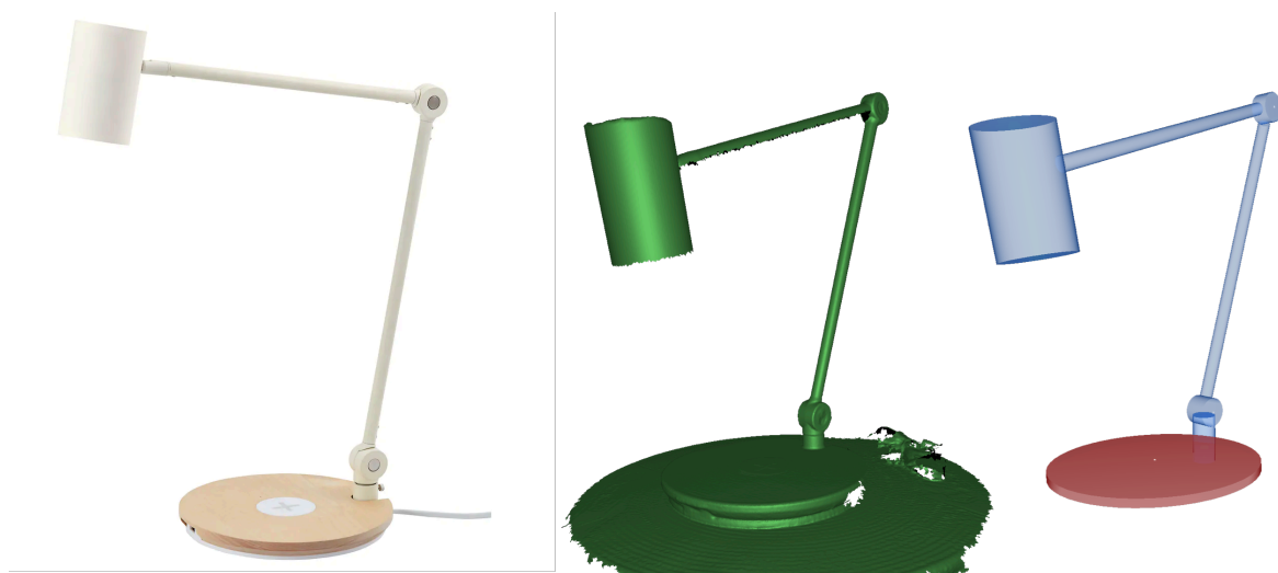
Figure 195: From left to right: original object, scanned model, a set of constructed primitives.
