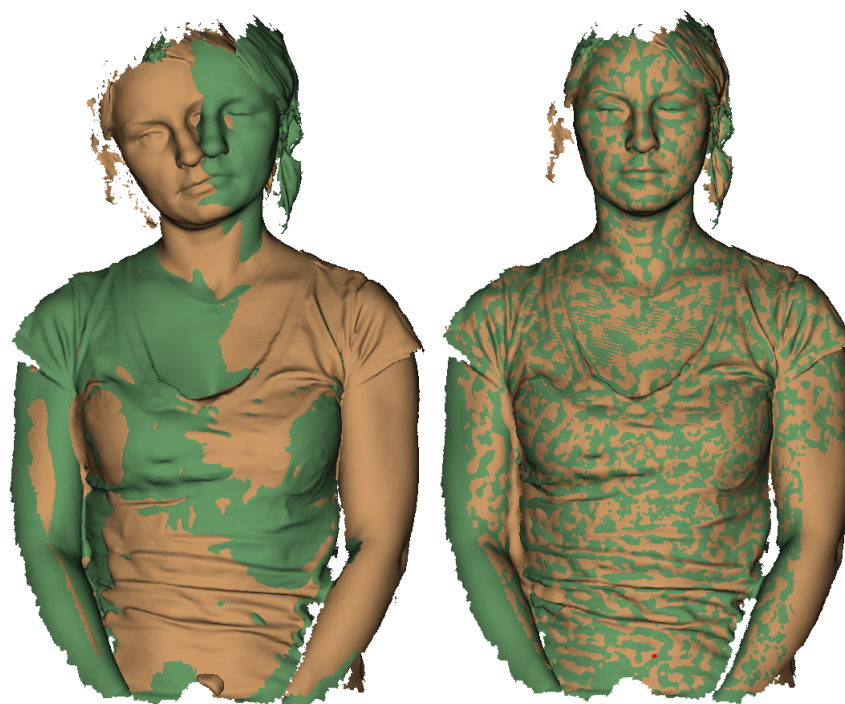
Figure 142: Two models after Best Fit (left) and nonrigid alignment (right).
