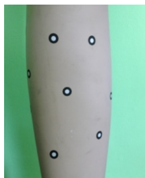
Figure 56: Non-coded targets placed on an object.
